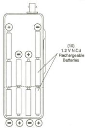
Nickel-cadmium battery placement
